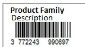
In this sample, we use the Code128 code. The label is made of 3 lines, from top to bottom. The text, which appears under the barcode is the barcode value.
